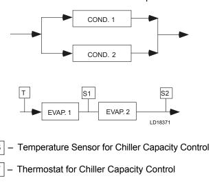
FIGURE 2 - SERIES EVAPORATORS PARALLEL CONDENSERS
