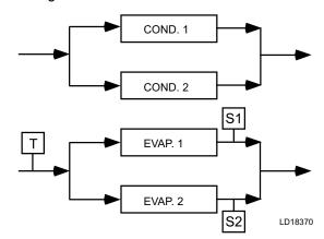
S - Temperature Sensor for Chiller Capacity Control
