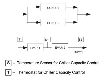
FIGURE 2 - SERIES EVAPORATORS PARALLEL CONDENSERS
