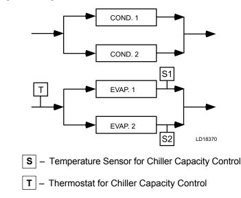
FIGURE 1 - PARALLEL EVAPORATORS PARALLEL CONDENSERS
