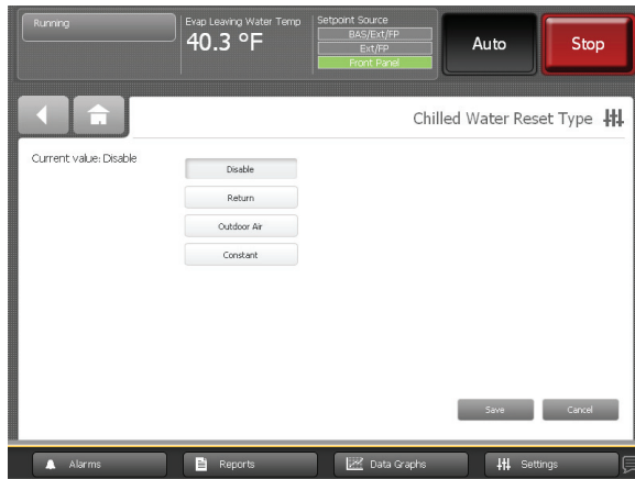
Figure 41. Chilled water setpoint screen
