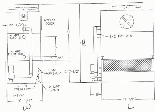
**Note:** The number of coil connections doubles when the flow rate exceeds 425 GPM on Models ATW 24-3G thru ATW 24-5G.
