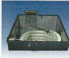
Coaxial evaporator inside the tank
