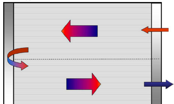
Figure 4: Typical 2-Pass Construction
