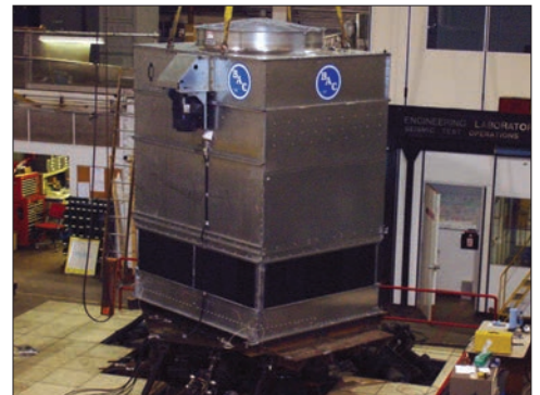
PT2 During Shake Table Testing
