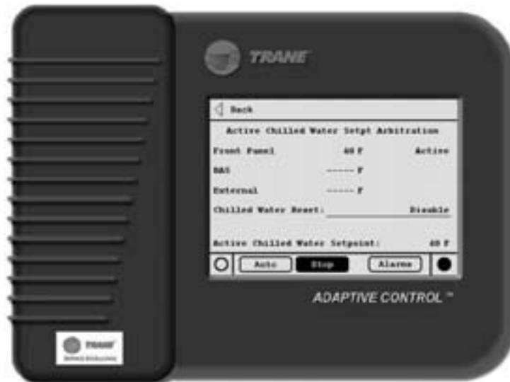
The **active chilled water setpoint** is the setpoint that is currently in use. It will be displayed to 0.1 degrees Fahrenheit or Celsius. Touching the **double arrow** to the left of the Active Chilled Water Setpoint will take the user to the active chilled water setpoint arbitration sub-screen.
