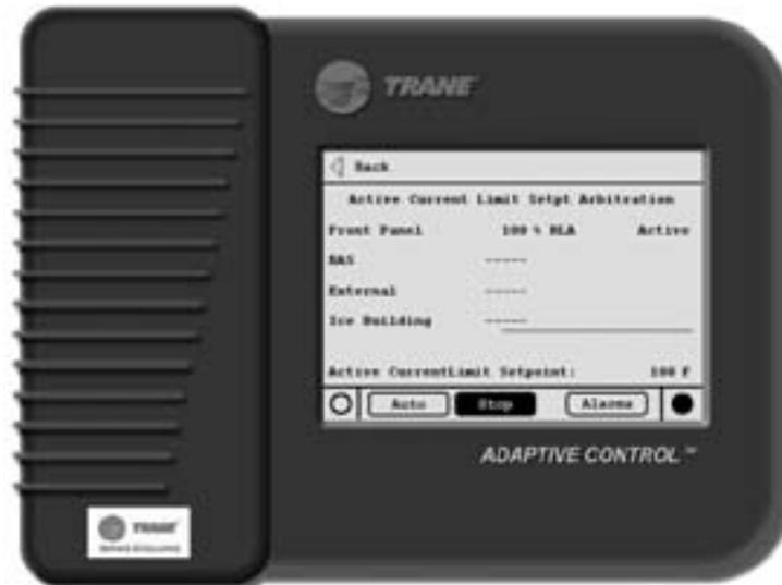
The **active current limit setpoint** is the current limit setpoint that is currently in use. It will be displayed in percent RLA. Touching the double arrow to the left of the Active Current Limit Setpoint will take the user to the active current limit setpoint sub-screen. The active current limit setpoint is that setpoint to which the unit is currently controlling. It is the result of arbitration between the front panel, BAS, and external setpoints.
