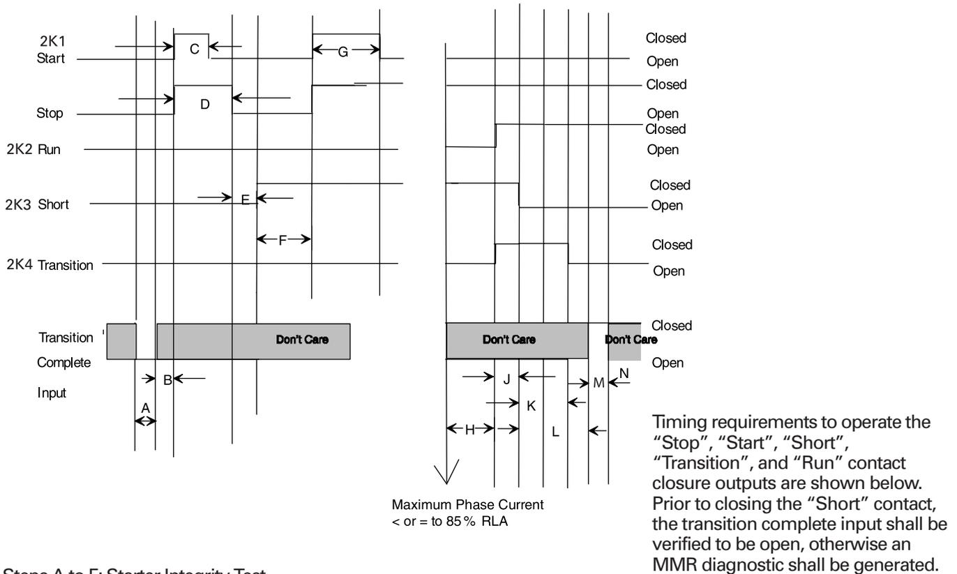
Steps A to F: Starter Integrity Test.
