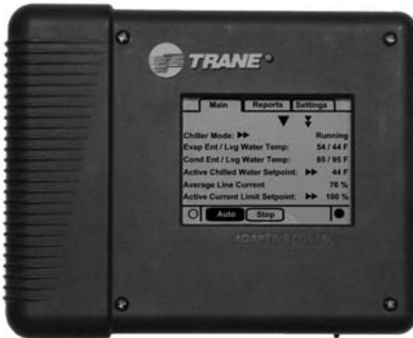
The **machine-operating mode** indicates the operational status of the chiller. A subscreen with additional mode summary information will be provided. When the user scrolls down the screen the Machine Operation Mode will remain stationary
