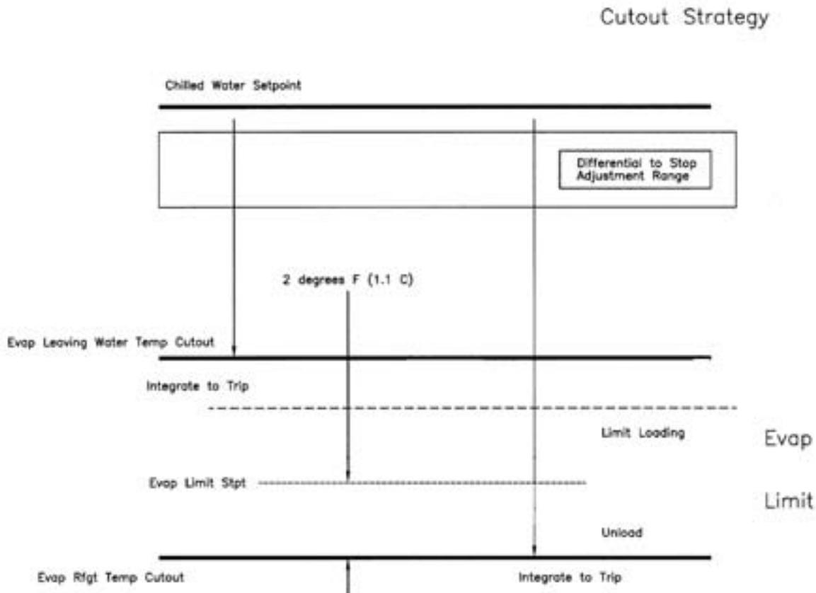
Limit Loading: The potential to limit loading increases as the saturated evaporator temperature approaches the evaporator limit setpoint.
