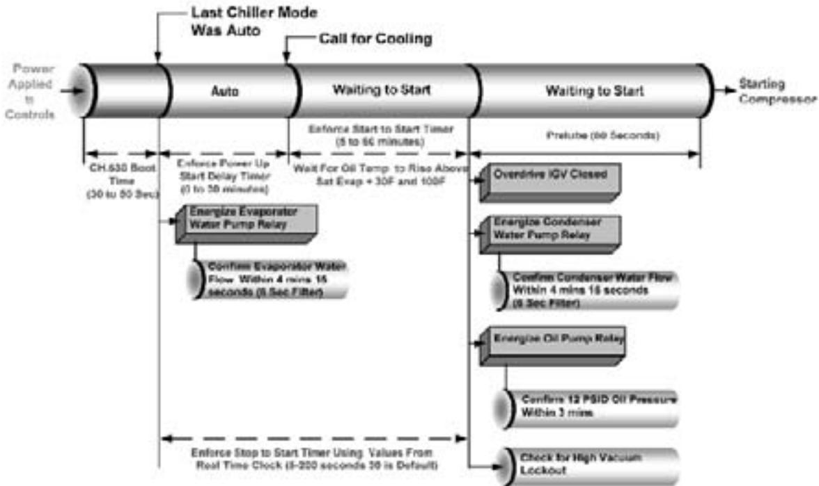
Figure 9. CVHE, CVHF, and CVHG sequence of operation: running
