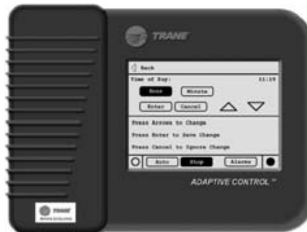
**Note:** The 24-hour format setpoint screen is similar with the am and pm not shown.
