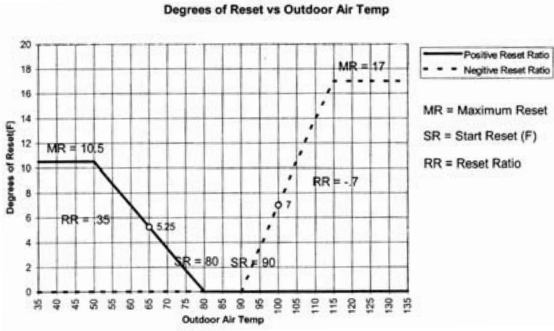
Figure 30. Reset function for return CWR
