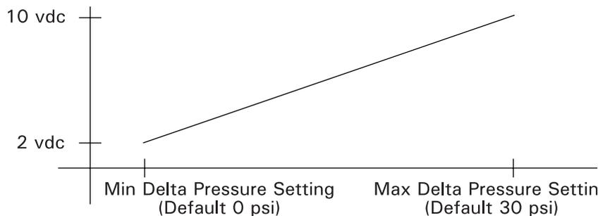
In this example, 2 vdc corresponds to 0 psi differential and 10 vdc corresponds to 30 psi differential. The min value of 0 psi, to the max value of 30 psi are individually adjustable via the service tool.
