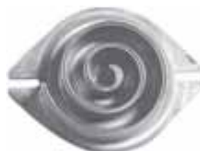
Figure 1. One of two matched scroll plates - the distinguishing feature of the scroll compressor
