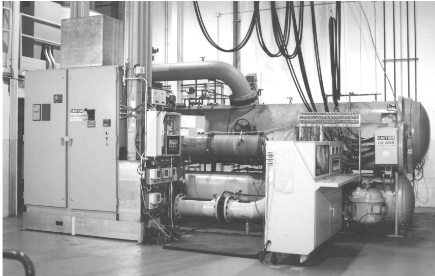
Figure 8 , McQuay’s million dollar compressor test stand with advanced data acquisition provides comprehensive information on new compressor designs.
